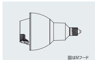
電球型LED **Mavros®-Cross-Beam** 色温度:L27=2700K L30=3000K W=4000K
